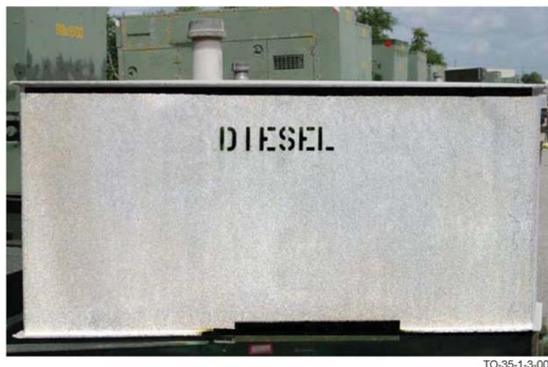
**Figure 1-6. Example of Uniform Etch**
