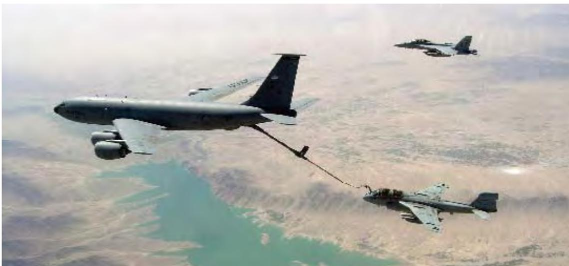
**High above Helmand Province, an Air Force KC-135R aerial tanker refuels a Navy EA-6B electronic warfare aircraft (bottom) and F/A-18 fighter. The Air Force’s capacity to gas up the aircraft of all services has been vital in Afghanistan. (DOD photo/Navy Cmdr. Erik Etz)**
