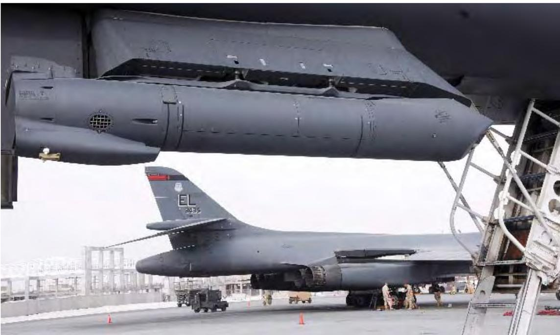
**In foreground, a Sniper advanced targeting pod hangs from the underside of a B-1B bomber. Another B-1B is shown in the background. With the Sniper pod, the B-1B can rapidly switch into its so-called "ISR mode" and monitor the battle space. (USAF photo/SSgt. Darnell Cannady)**
