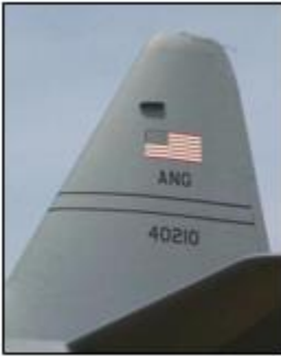
Figure A3.1. C-130 & C-27 Equipment Excellence Gray Tail Scheme and Standard Markings.
