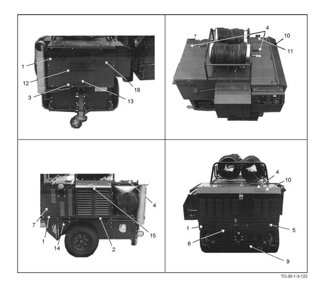
Figure 4-53. New Generation Heater (Sheet 1 of 3)
