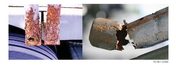
Figure 1-3. Corrosion Accelerated by Condensed Moisture
