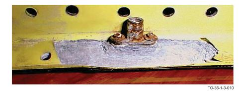
Figure 1-10. Example of Exfoliation Corrosion
