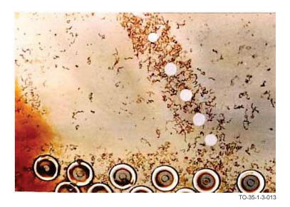
Figure 1-13. Example of Filiform Corrosion
