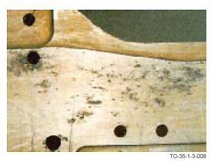
Figure 1-8. Example of Pitting Corrosion
