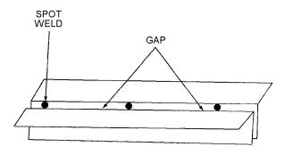
STRUCTURAL STEEL (ANGLE IRON) T GAPS/SEAMS TO-35-1-3-125
