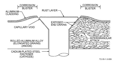
Figure 1-9. Illustration of an Intergranular Corrosion Cell
