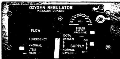
Two manufacturers produce CRU-73 Oxygen Regulators. Both offer same BIT capability, but accomplish it in slightly different ways. With Bendix regulator (shown here), only a portion of OXYGEN mixture toggle moves to 100% oxygen when you turn SUPPLY toggle OFF. With ARO regulator, entire toggle moves. Incidentally, you can identify CRU-73 Regulator through the two test ports on either side of the pressure gage (CRU-68 does not have test ports, and SUPPLY toggle is safety-wired to ON position).
