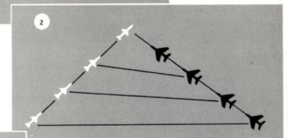
INCORRECT MISSILE HEADING RESULTING IN LARGE MISS. (NO MISSILE CORRECTION IN RESPONSE TO CHANGING TARGET-TO-MISSILE LINE OF SIGHT.)
