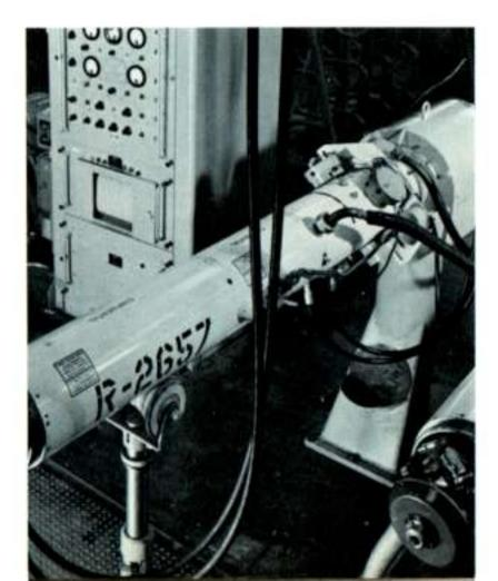
FIRE CONTROL SYSTEM — To facilitate maintenance, the fire control system test equipment is designed to isolate and replace a defective unit without removing the system from the aircraft. Testing and maintenance are divided into four levels as follows:
