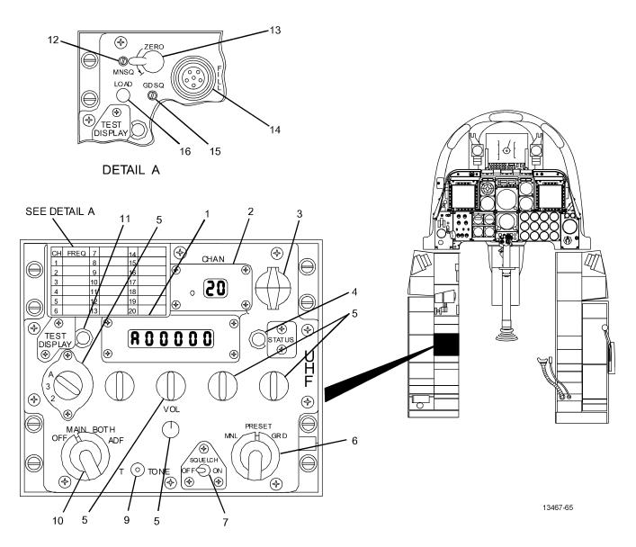
Figure 1-113. Have Quick II (HQII) UHF Radio RT-1505A/C/ARC-164(V) (Sheet 1 of 4)
