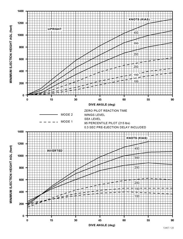
Figure 3-4. Minimum Ejection Altitude vs Dive Angle and Speed
