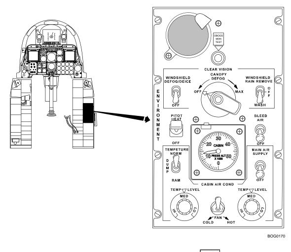
Figure 1-30.1. Environment Control Panel 518
