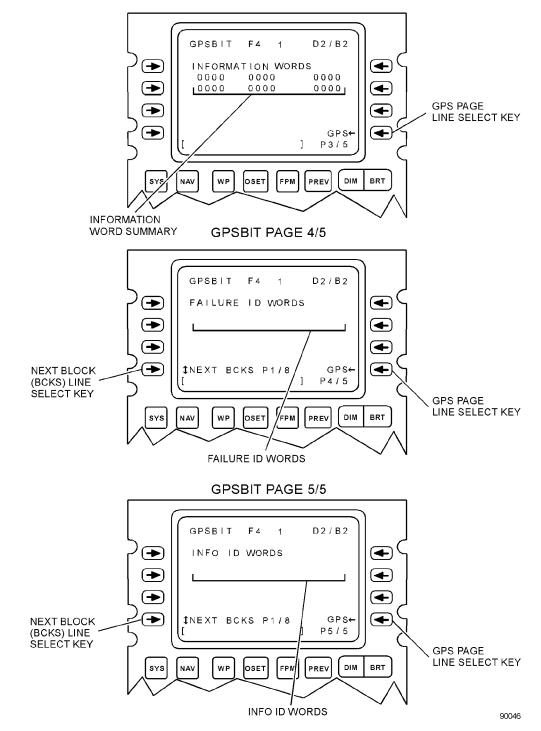
Figure 1-96. GPS BIT (GPSBIT) Pages (Sheet 2)
