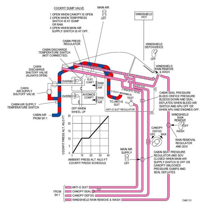
Figure 1-29. Environment System Schematic (Sheet 2)
