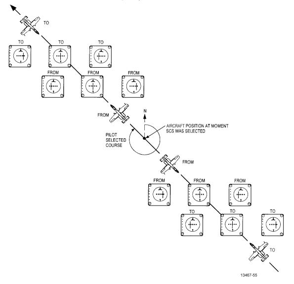
Figure 1-55. Horizontal Steering (2D or 3D Mode) (Sheet 4)
