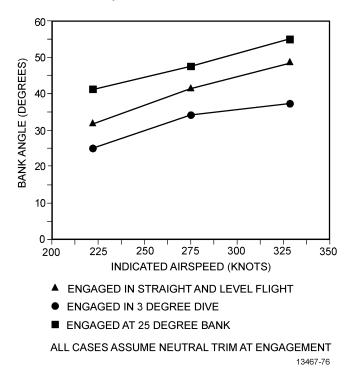
Figure 1-183. Typical Altitude/Bank Hold Envelope for 5000 Feet
