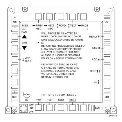
Figure 1-140.6. Message Page (Sample Text Receipt) (Sheet 1 of 4)
