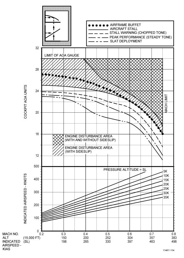
Figure 6-2. Stall Warning and Engine/Airframe Compatibility
