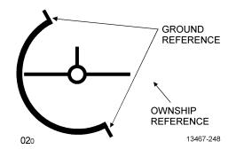
Figure 1-165. ARS Components (Displayed in Straight Flight With 45° Left Bank)
