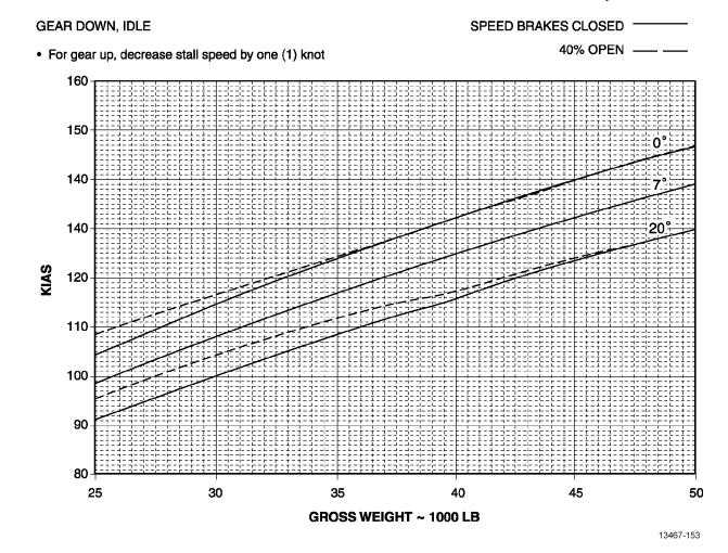
Figure 6-1. In-Flight Stall Speeds
