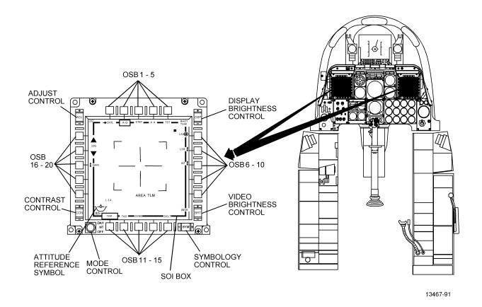
Figure 1-164. Multifunction Color Displays (MFCDs)
