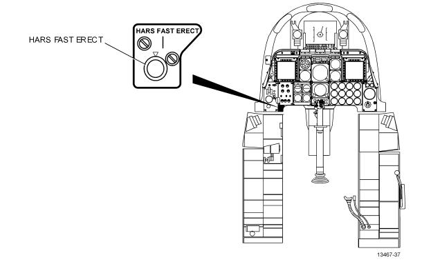
Figure 1-36. HARS Fast Erect Switch
