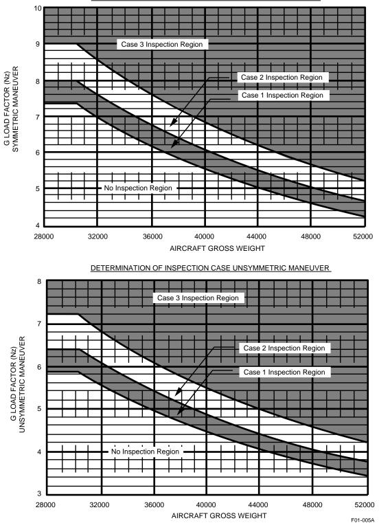
DETERMINATION OF INSPECTION CASE SYMMETRIC MANEUVER
