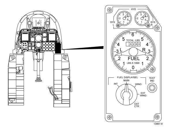
Figure 1-8. Fuel Quantity Indicator and Selector
