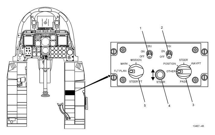
Figure 1-50. Avionics Auxiliary Panel (Sheet 1 of 2)
