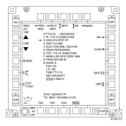
Figure 1-152.10. MA Message View Page (Sample Transmitted VMF MA Message)
