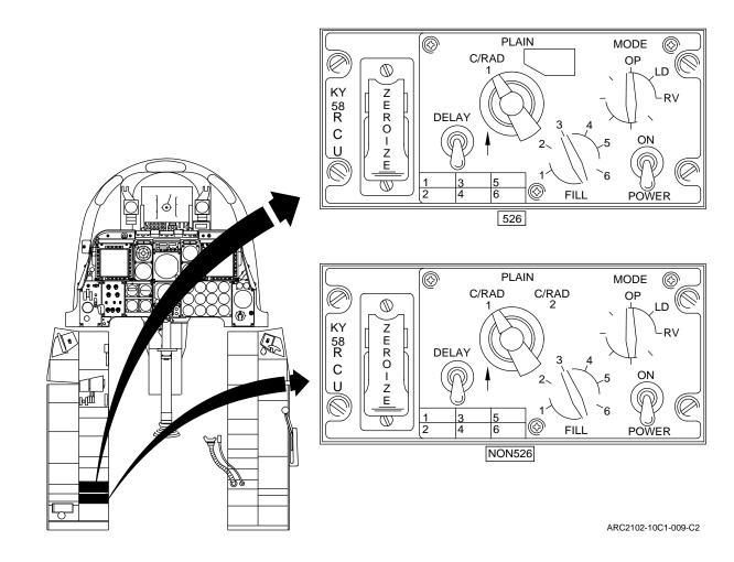
Figure 1-115. Secure Voice Control Panel
