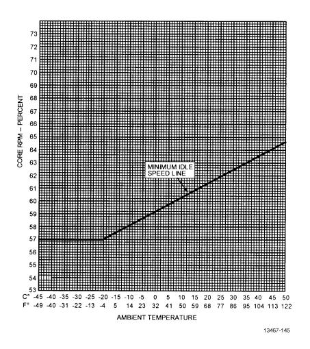
Figure 5-4. Minimum Idle Speed Core Percent RPM Limits
