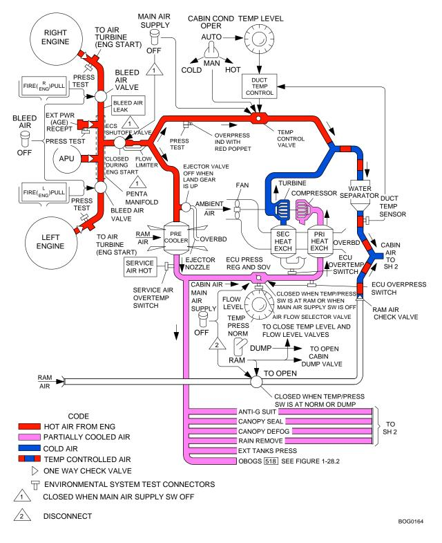
Figure 1-29. Environment System Schematic (Sheet 1 of 2)
