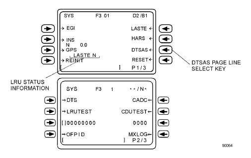
Figure 1-80. System (SYS) Pages (Sheet 1 of 3)
