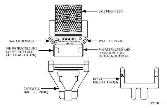
Figure 1-25. Universal Water Activated Release System (UWARS)
