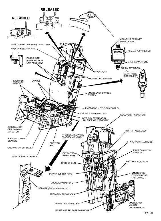
Figure 1-24. ACES II Ejection Seat
