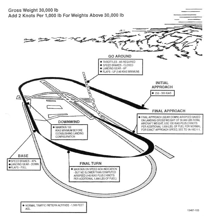
Figure 2-7. Typical Overhead Landing Pattern
