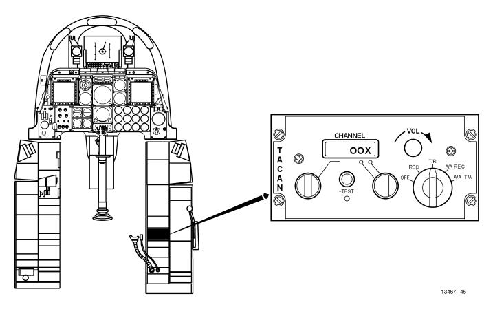
Figure 1-45. TACAN Control Panel - AN/ARN-118(V) (Sheet 1 of 2)
