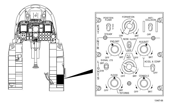
Figure 1-157. Lighting Control Panel
