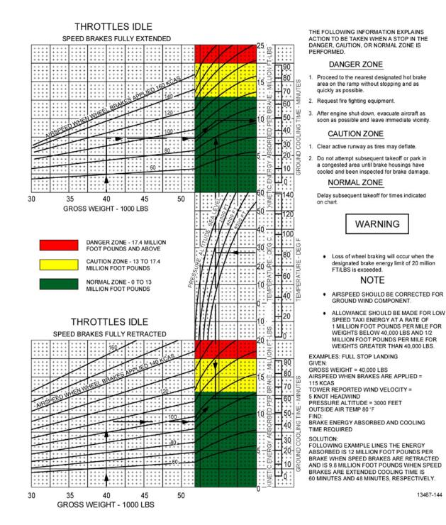
Figure 5-3. Wheel Brake Energy Limits (One Continuous Brake Application)
