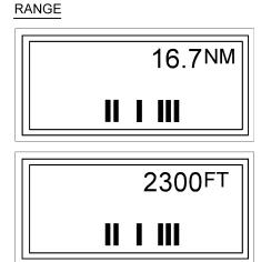
Range to survivor displayed in nautical miles to the nearest 0.1 mile until within 9999 feet, then range is displayed in feet (100's of feet from 9900 to 1000, 10's of feet from 990 to 0). If four dashes are displayed, no range value has been received.
