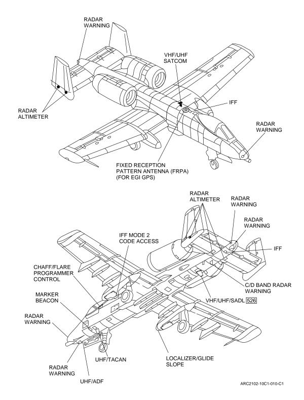
Figure 1-43. Antenna Locations (Sheet 2)
