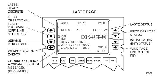
Figure 1-82. LASTE Page (Sheet 1 of 3)
