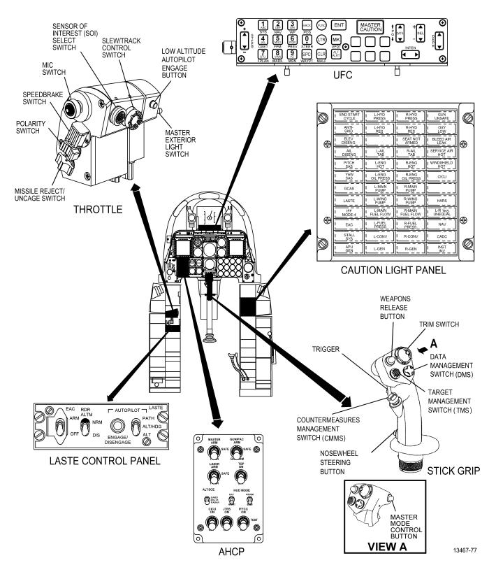
Figure 1-184. LASTE Cockpit Interfaces
