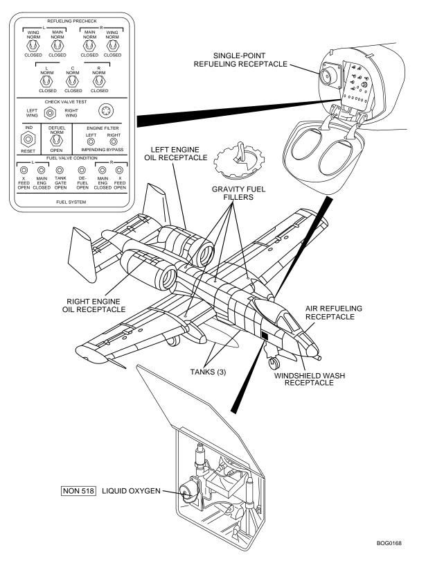
Figure 1-204. Servicing Diagram (Sheet 1 of 5)
