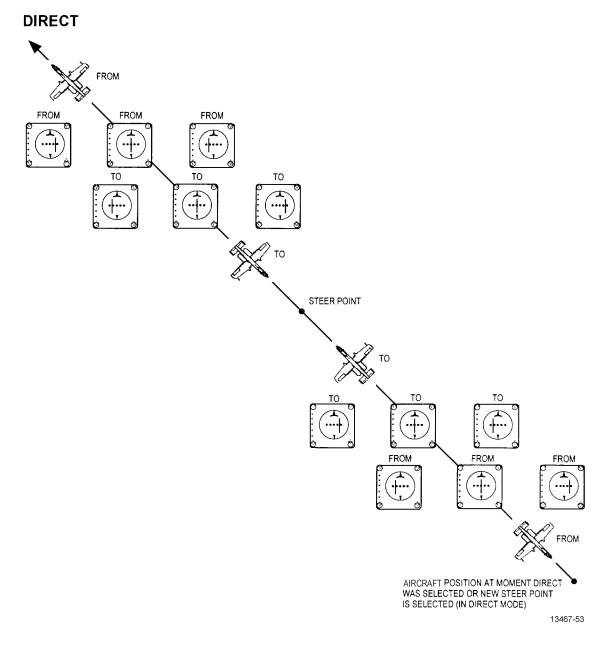
Figure 1-55. Horizontal Steering (2D or 3D Mode) (Sheet 2)
