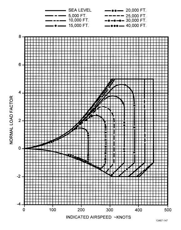
Figure 5-5. Flight Strength Diagram (Sheet 2)
