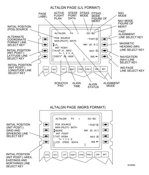
Figure 1-90. Alternate Align (ALTALGN) (Sheet 1 of 5)
