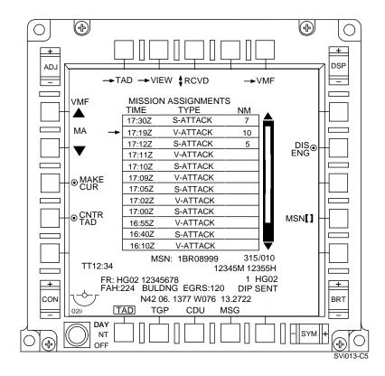
Figure 1-152.13. VMF Mission Assignment Status Displayed on TAD MA Page
