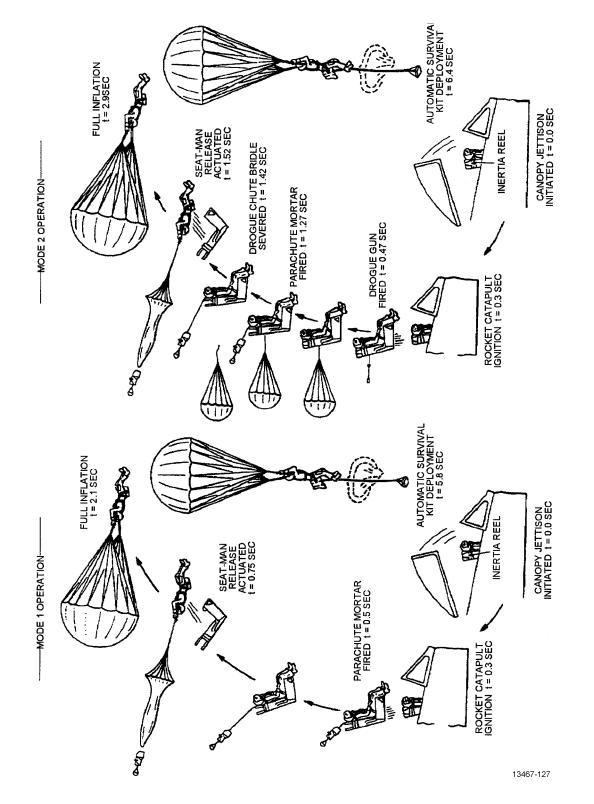
Figure 3-5. Ejection Seat Operation
