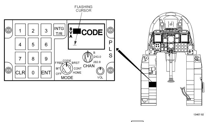
Figure 1-202. LARS Control Display Unit (CDU) 131 (Sheet 1 of 2)
