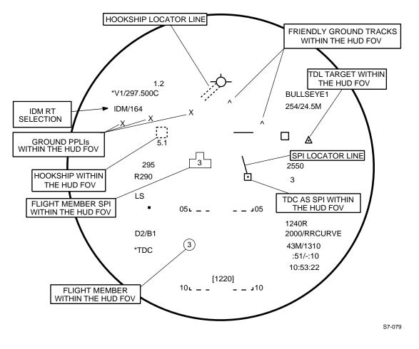
Figure 1-140.2. HUD Display (Data Link Symbols in FOV)
