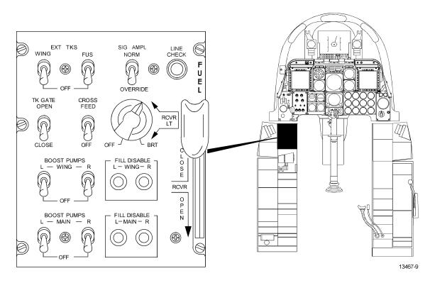
Figure 1-9. Fuel System Control Panel
