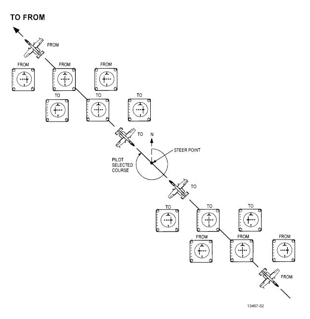
Figure 1-55. Horizontal Steering (2D or 3D Mode) (Sheet 1 of 4)
