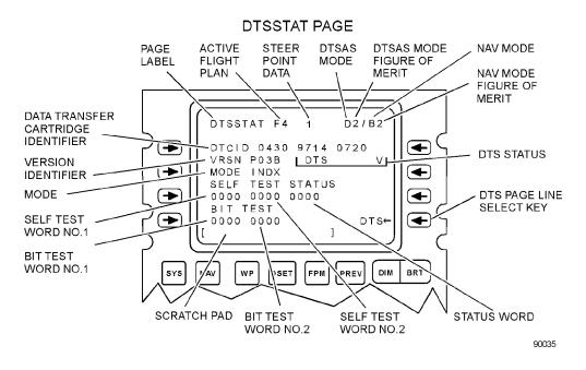
Figure 1-100. DTS Status (DTSSTAT) Page (Sheet 1 of 2)
