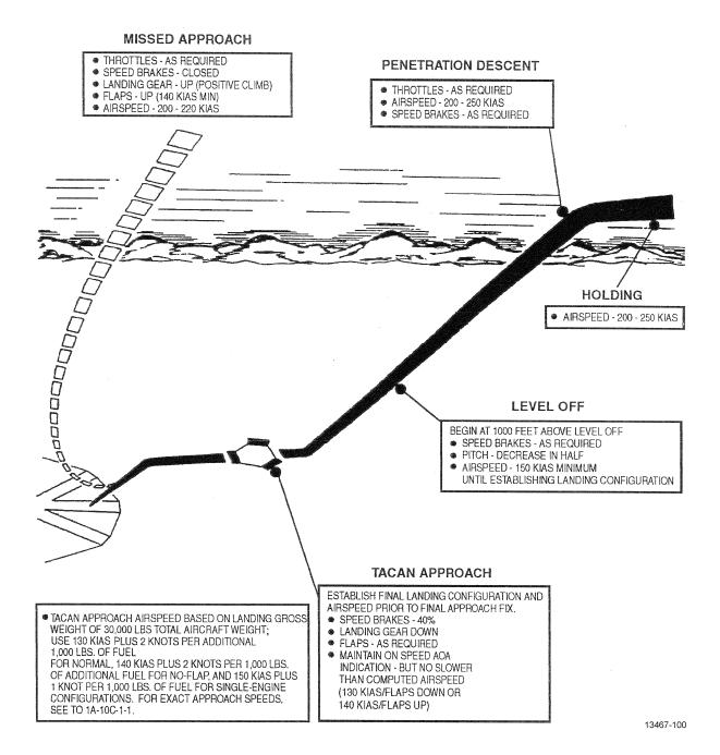
Figure 2-4. TACAN Penetration and Approach - Typical
