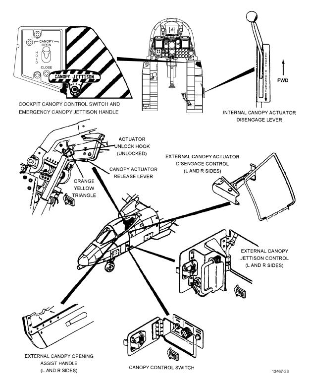
Figure 1-23. Canopy Controls (Sheet 1 of 2)
