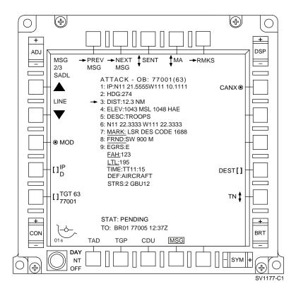
Figure 1-153. MA Message View Page (Sample Transmitted MA Message)
