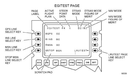
Figure 1-102. EGI Test (EGITEST) Page (Sheet 1 of 2)
