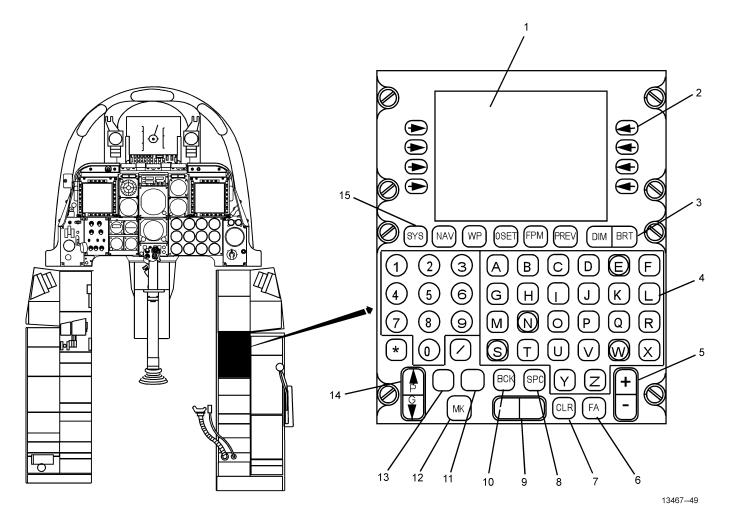
Figure 1-51. Control Display Unit (Sheet 1 of 4)
