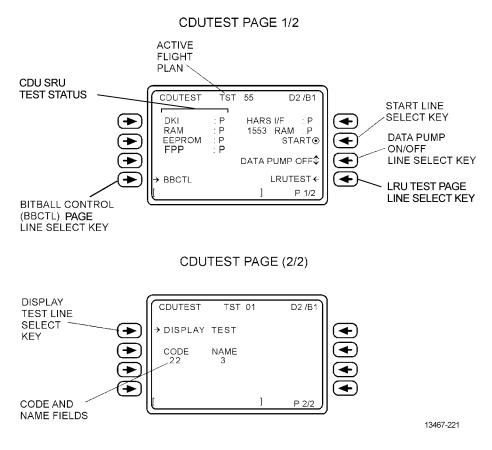
Figure 1-103. CDU Test (CDUTEST) Pages (Sheet 1 of 2)
