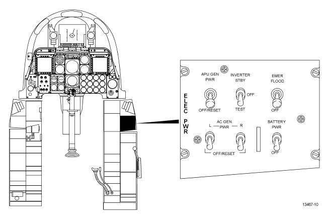
Figure 1-10. Electrical Power Control Panel
