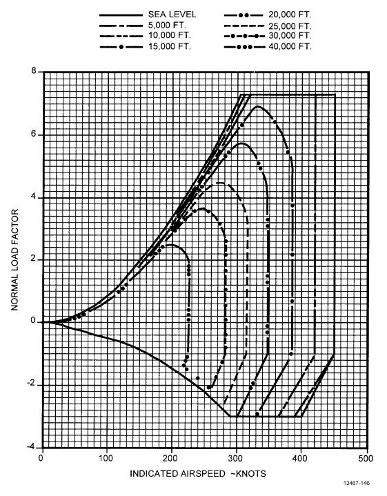
Figure 5-5. Flight Strength Diagram (Sheet 1 of 3)
