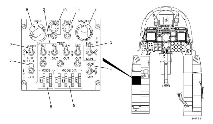
Figure 1-111. IFF/SIF Control Panel (Sheet 1 of 3)
