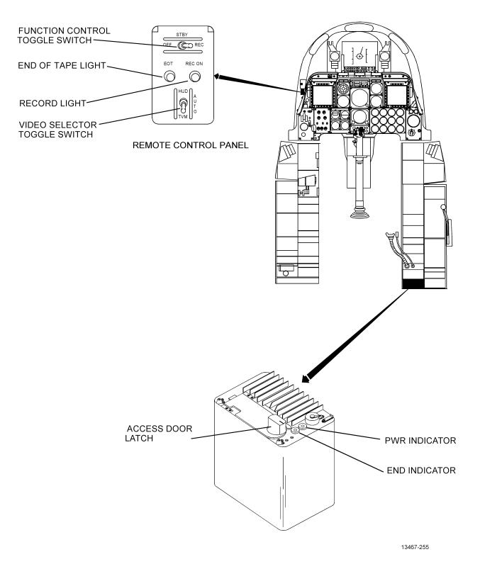
Figure 1-201. Color Cockpit Television Sensor (CCTVS)/Digital Video Airborne Data Recorder (DVADR) (Sheet 1 of 2)
