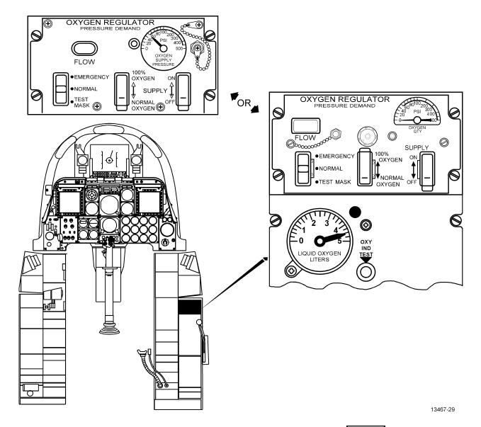
Figure 1-28. Oxygen System Regulator and Quantity Gauge NON518
