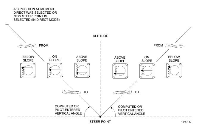
Figure 1-56. Vertical Steering (3D Mode Selected) (Sheet 2)
