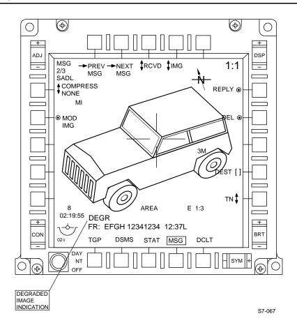
Figure 1-140.4. Degraded Image Message Page (Sample Received SADL IMG)
