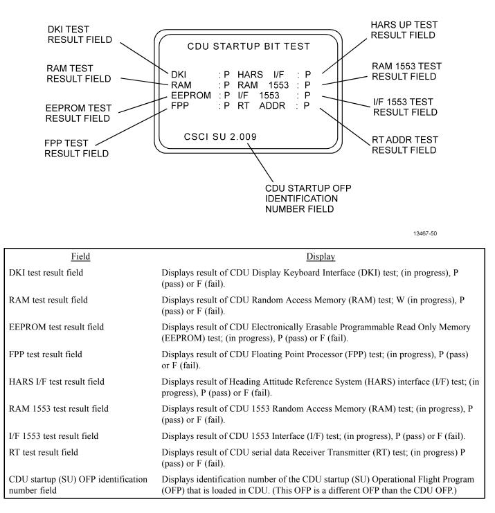
Figure 1-52. CDU Startup BIT Test Display
