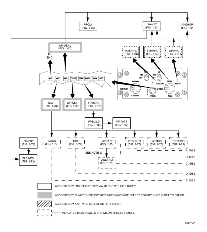
Figure 1-57. ENAV CDU Display Pages Menu Tree (Sheet 1 of 2)
