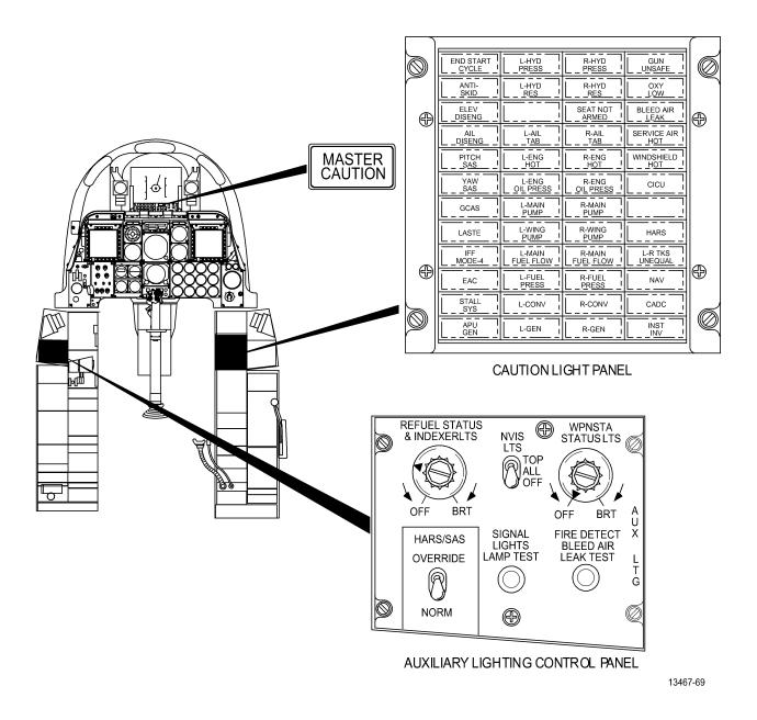
Figure 1-158. Caution Light Panel and Auxiliary Lighting Control Panel
