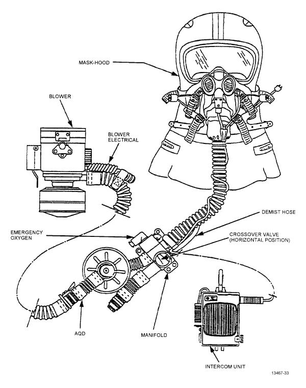
Figure 1-32. Aircrew Eye/Respiratory Protection (AERP) System
