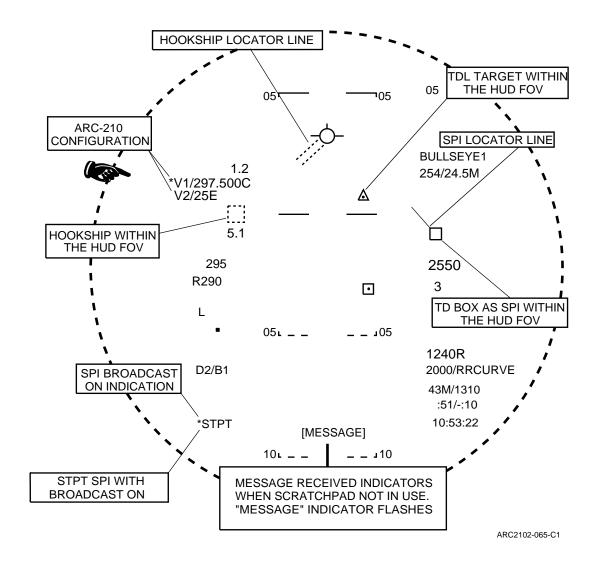
Figure 1-140.1. HUD Display (Message Indication, No Data Link Symbols in FOV)
