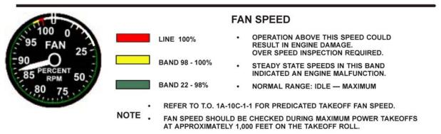
• THE 1% BELOW MINIMUM TRIM AUTHORIZED FOR SELECTED TF34-GE-100 ENGINES, SHALL NOT BE A FACTOR WHEN COMPUTING TAKEOFF FAN SPEED.
