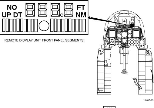
Figure 1-203. LARS Remote Display Unit (RDU) 131 (Sheet 1 of 3)
