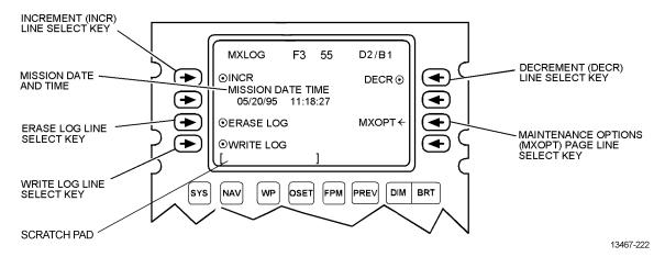
Figure 1-108. Maintenance Log (MXLOG) Page (Sheet 1 of 2)
