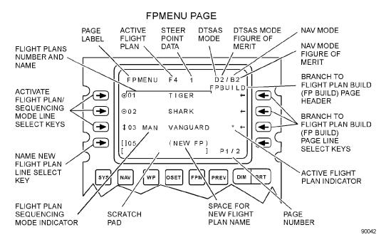
Figure 1-67. Flight Plan Menu (FPMENU) Page(s) (Sheet 1 of 3)
