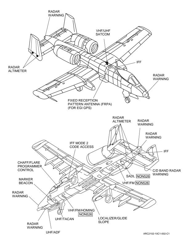
Figure 1-43. Antenna Locations (Sheet 1 of 2)
