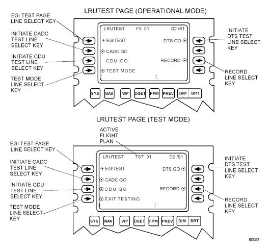
Figure 1-101. LRU Test (LRUTEST) Page (Sheet 1 of 2)
