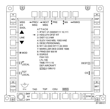
Figure 1-140.7. MA Message Page (Sample Pre-canned MA)
