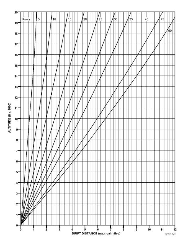
Figure 3-6. Parachute Drift Distance vs Altitude
