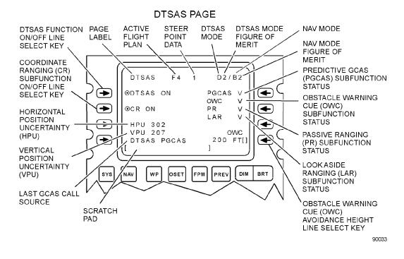
Figure 1-93. Digital Terrain System Application Software (DTSAS) Page (Sheet 1 of 3)
