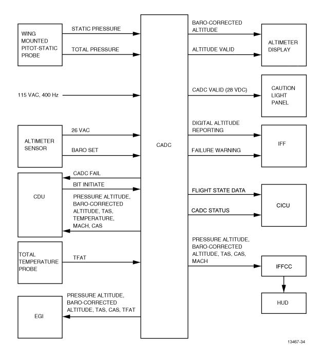
Figure 1-33. Central Air Data Computer Interfaces
