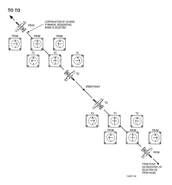
Figure 1-55. Horizontal Steering (2D or 3D Mode) (Sheet 3)
