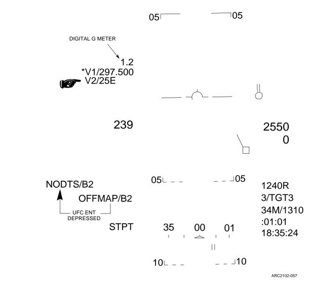
Figure 1-181. "OFFMAP" Error Message and Digital G Meter
