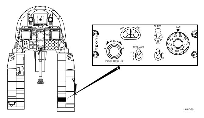
Figure 1-35. Heading Attitude Reference System Control Panel (Sheet 1 of 2)
