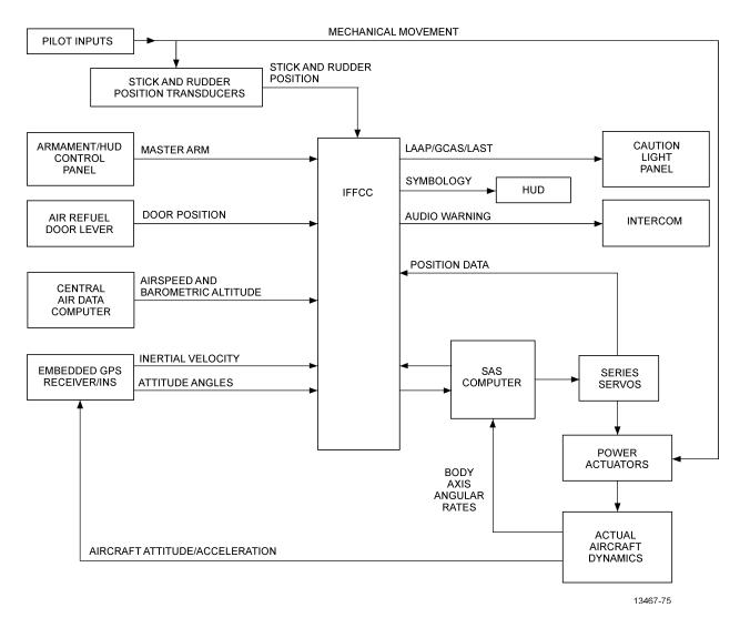
Figure 1-182. Enhanced Attitude Control (EAC) System Tie-In
