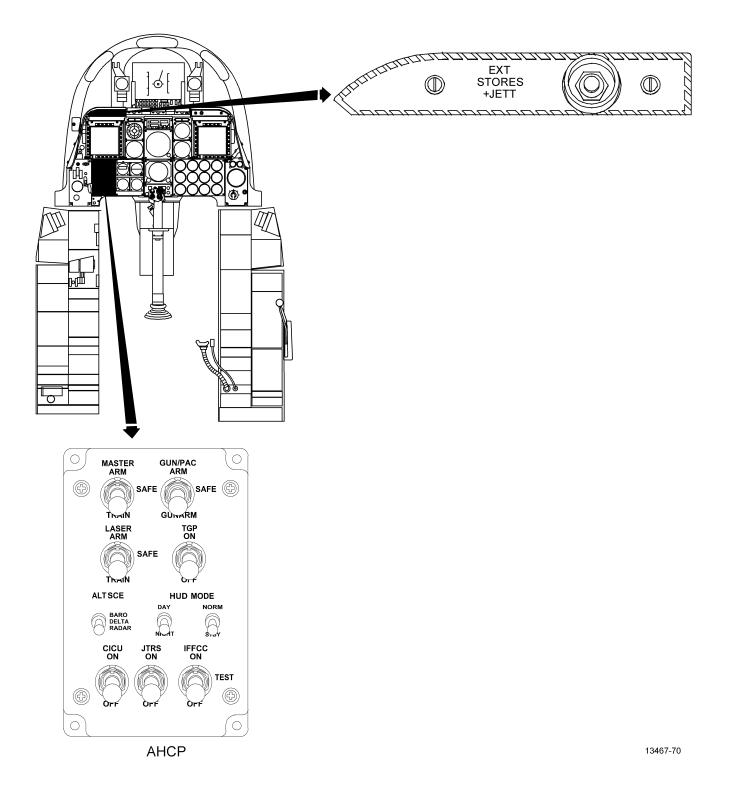
Figure 1-174. Armament System Controls (Sheet 1 of 2)
