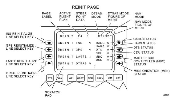
Figure 1-81. Reinitialization (REINIT) Page (Sheet 1 of 2)
