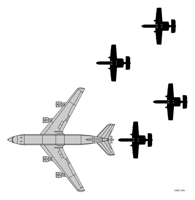
Figure 2-16. Quick Flow Air Refueling
