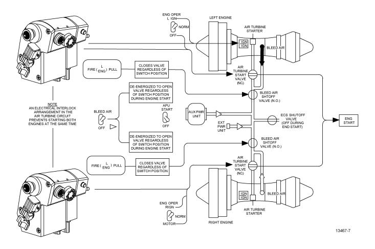
Figure 1-6. Engine Start System
