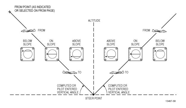
Figure 1-56. Vertical Steering (3D Mode Selected) (Sheet 3)
