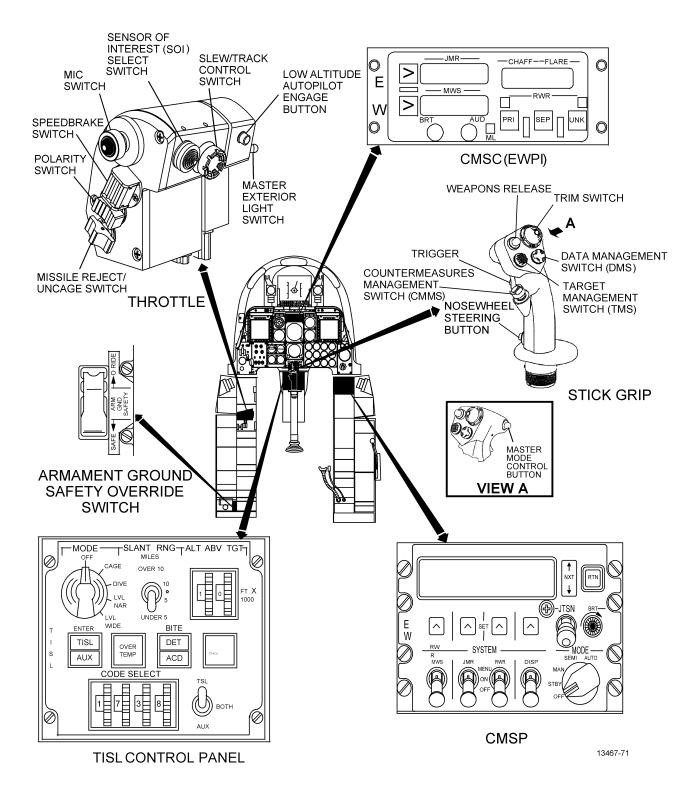
Figure 1-174. Armament System Controls (Sheet 2)
