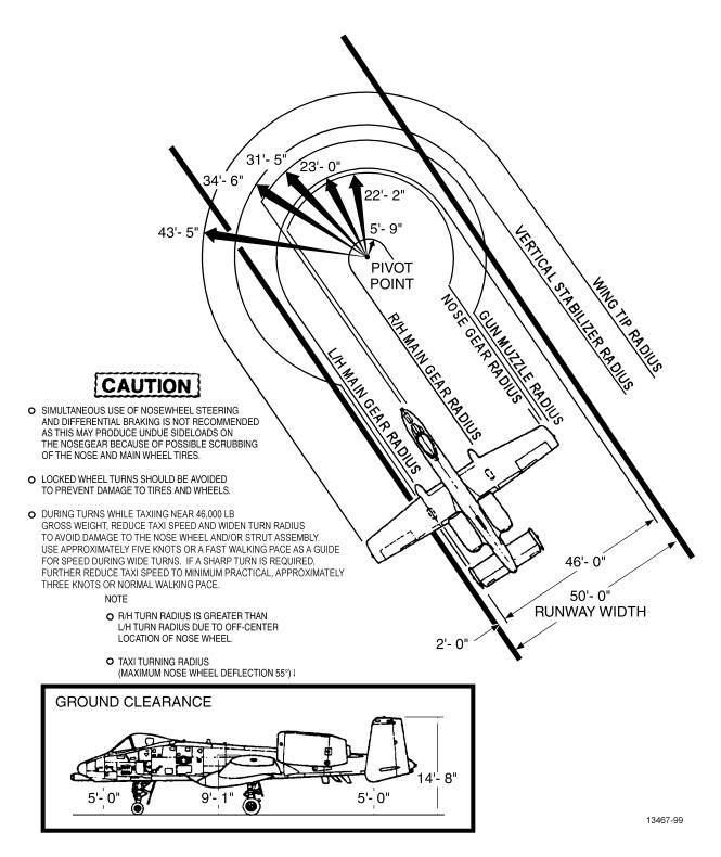
Figure 2-3. Turning Radius and Ground Clearance
