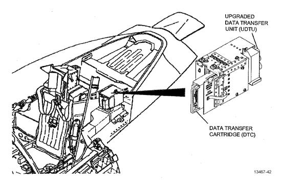
Figure 1-41. Data Transfer System (DTS)
