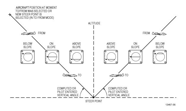
Figure 1-56. Vertical Steering (3D Mode Selected) (Sheet 1 of 4)
