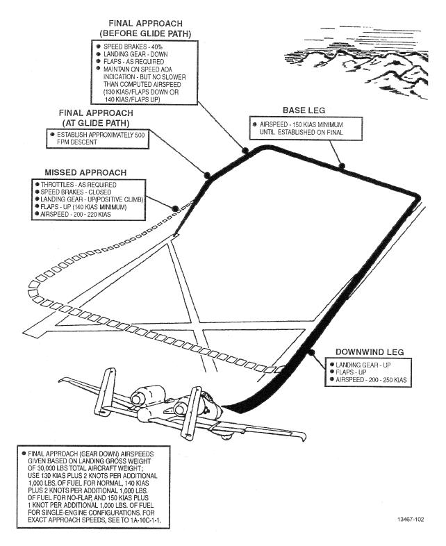
Figure 2-6. Typical Radar Approach - GCA
