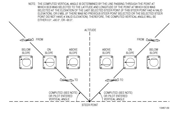
Figure 1-56. Vertical Steering (3D Mode Selected) (Sheet 4)
