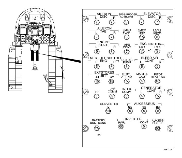
Figure 1-11. Circuit Breaker Panel (Sheet 1 of 2)
