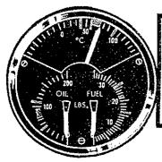
ENGINE GAGE UNIT FUEL PRESSURE INDICATOR
