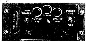
This equipment is not a complete system, but when used with the AN/ARC-156 or PM-622A radio it performs the encryption and decryption functions necessary to secure voice communications. The basic equipment consists of a unit installed in the aft fuselage and a control panel located on the aft control pedestal. Power is received through whichever radio is being used.
