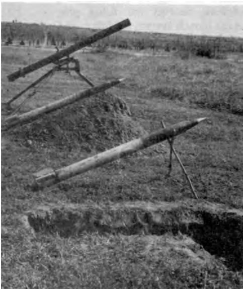
Display of the three basic methods used by the Viet Cong to launch rockets: launch tube, earth embankment, and crossed sticks
