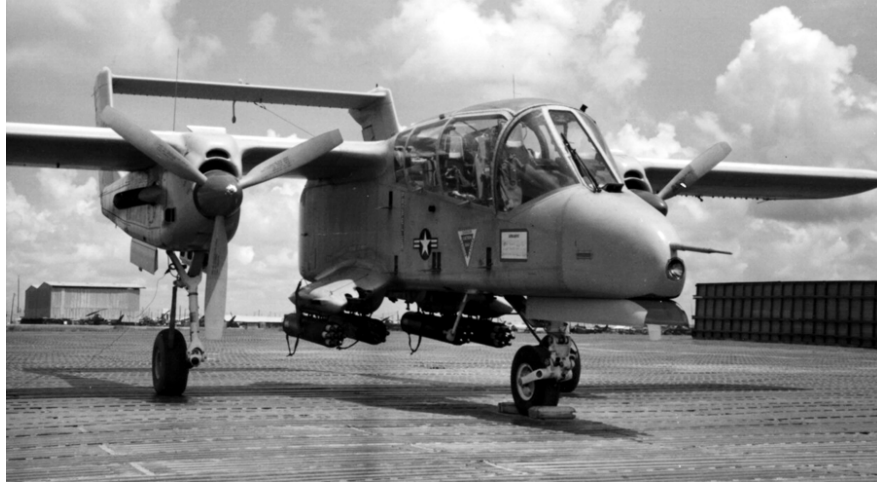
An OV-10 Bronco, with machineguns and rocket pods under the fuselage.
