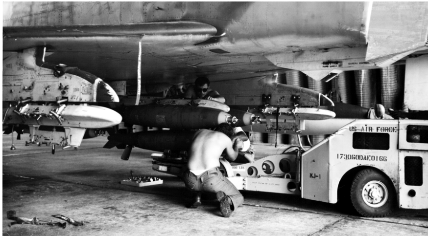
Airmen load 500-pound bombs on an F-4 at Phu Cat.
