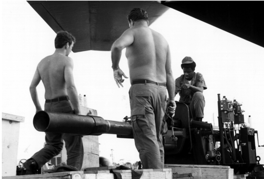
Armament personnel at Ubon Air Base, Thailand, inspect a 105-mm howitzer before installing it on an AC-130 gunship.
