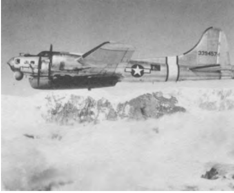
Left: SB-17 with a lifeboat attachment, flying over Alaska; center, SB-29 equipped with a drop boat for rescue; bottom: drop boat parachuting from an SB-29.
