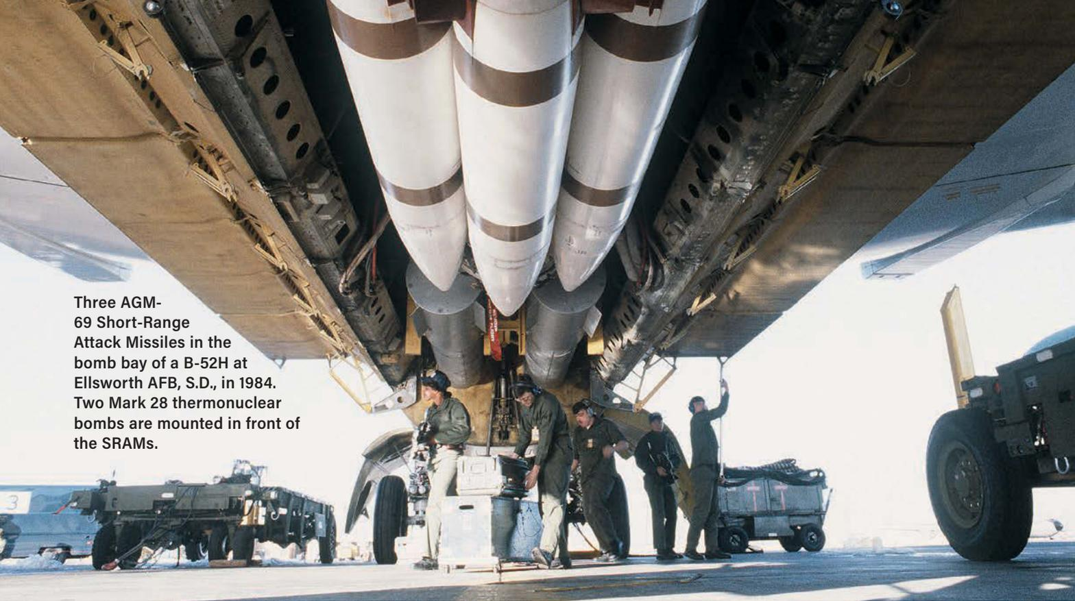
Three AGM-69 Short-Range Attack Missiles in the bomb bay of a B-52H at Ellsworth AFB, S.D., in 1984. Two Mark 28 thermonuclear bombs are mounted in front of the SRAMs.
