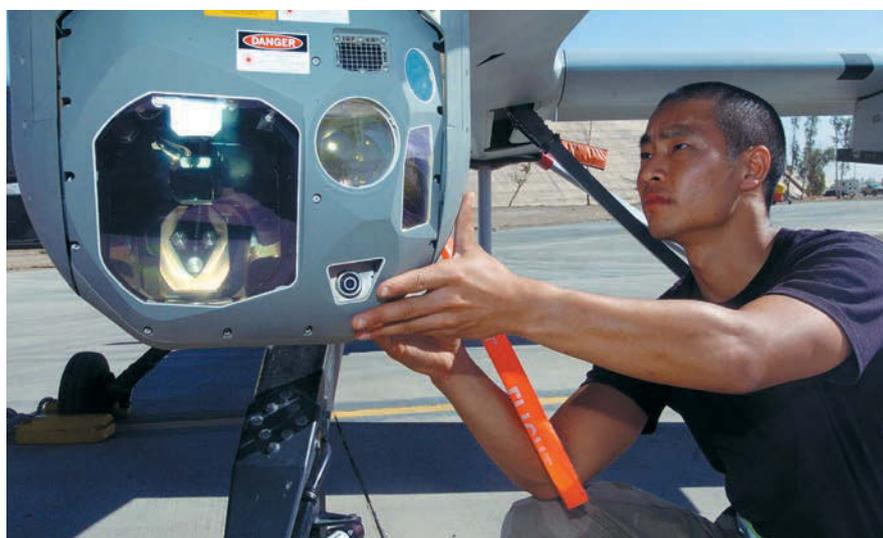
AIC Chris Korenaga checks the camera system of an RQ-1 Predator at Balad AB, Iraq. The unmanned aerial vehicle performed surveillance and reconnaissance patrols around the base's perimeter.
