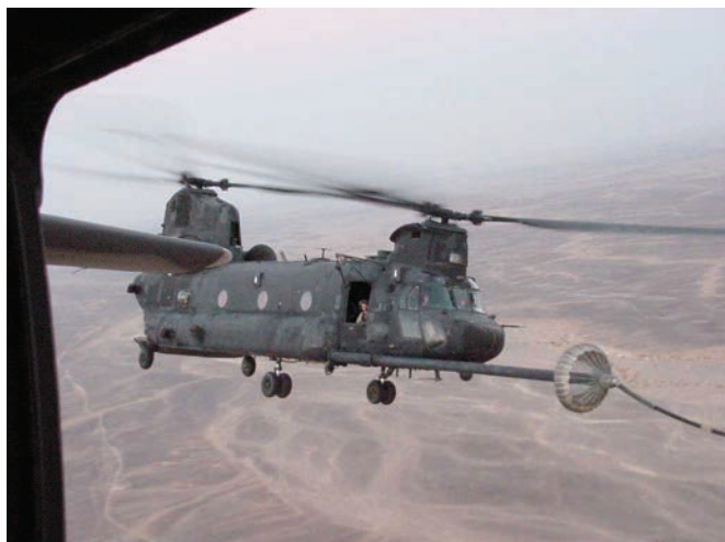
View from one the MC-130s as the receiver approached the drogue to onload fuel during EARLY VICTOR in October 2000. (Photo courtesy of the author)
