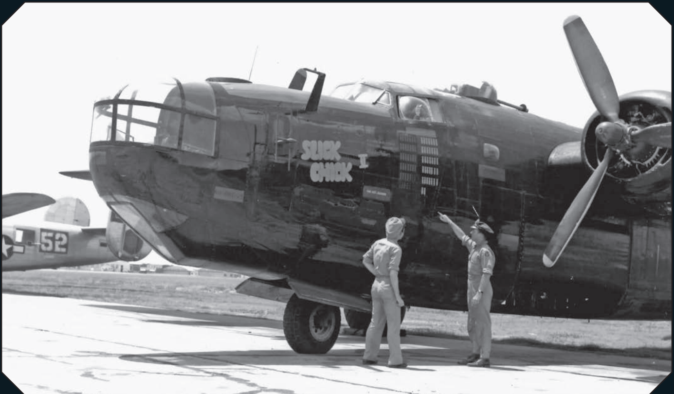
CARPETBAGGER B-24H with special modified navigator position in nose. (Photo courtesy of the Moore Collection)
