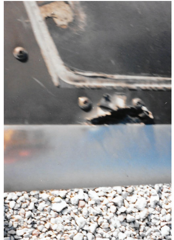
exit hole of bullet in mh-60 main rotor blade looking from top down. (Photo courtesy of Bill Denehan)
