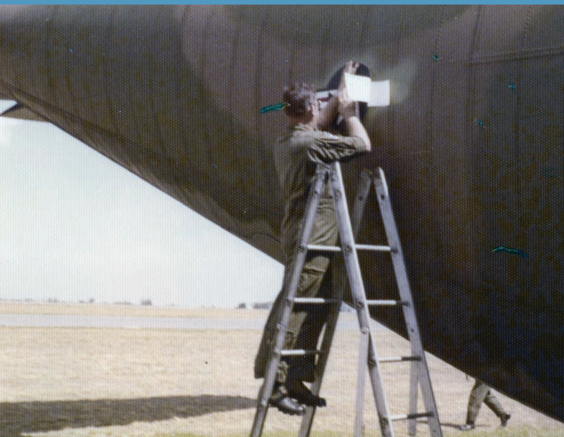
USAF decal being applied after VnAF markings have been sprayed out. (Photo courtesy of Bill Castlen)
