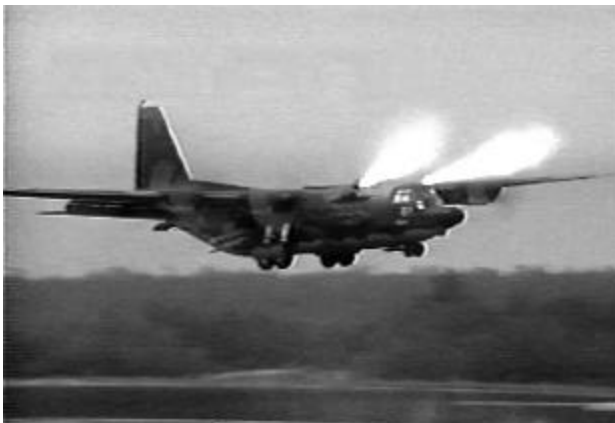
USAF Photo Aircraft 74-1683 begins its rocket-assisted maximum-effort landing. The top four reverse-mounted ASROC rockets have fired to slow the aircraft's forward flight vector.
